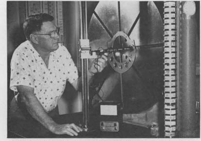
PRECISE MECHANICAL MEASUREMENTS are made by R. B. "Red" DeWitt (5523-3) to compare against specifications of the part. The measuring device is a Pla-Chek indicator which is accurate measuring distances within two seconds of one degree. partment manager, says, "QA continuously advises the AEC of the quality and reliability of stockpile weapons and notifies designers and producers of previously undetected problems which require correction."
